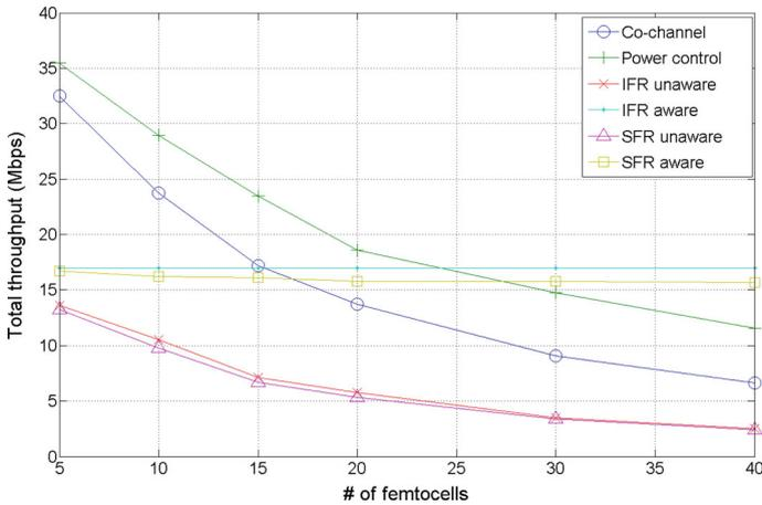
Fig. 16 Overall throughput performance for macro users for each ICIC at cell’s borders
