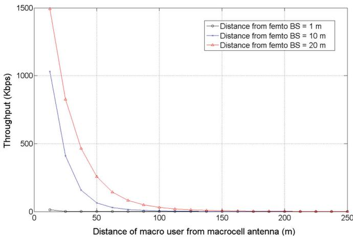
**Fig. 5** Throughput for an indoor macro UE against the distance from the macro BS when femtocell interference exists
