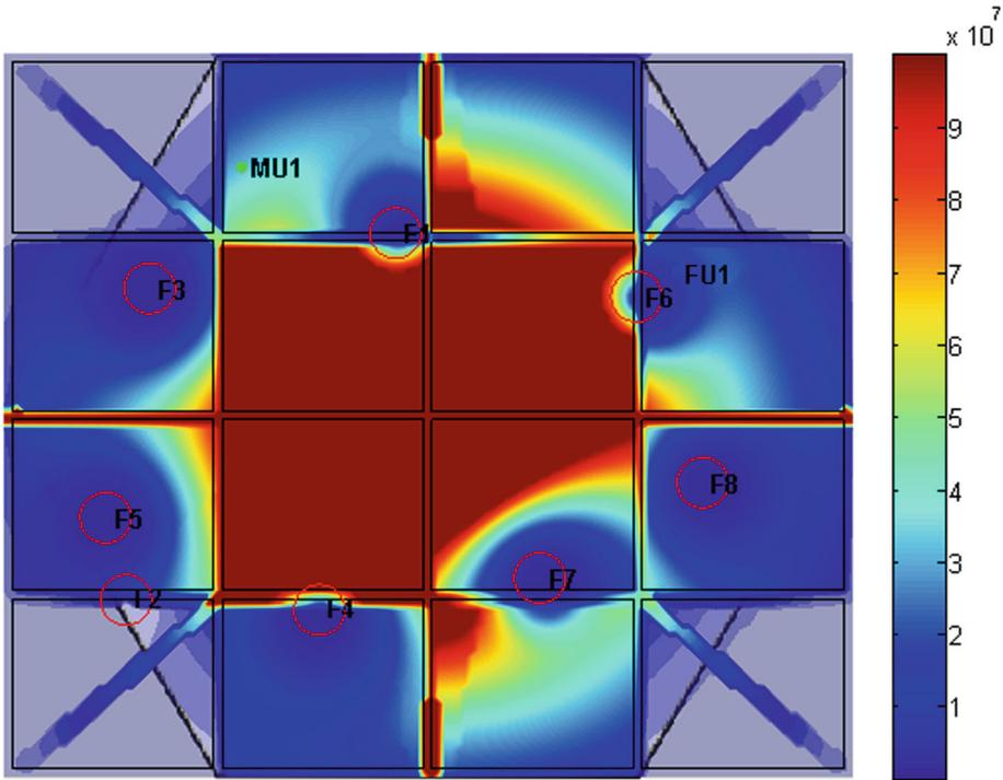
**Fig. 11** Throughput with power configuration for steady radius of service (macro user)
