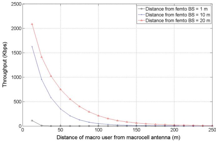
**Fig. 6** Throughput for an outdoor macro UE against the distance from the macro BS when femtocell interference exists
