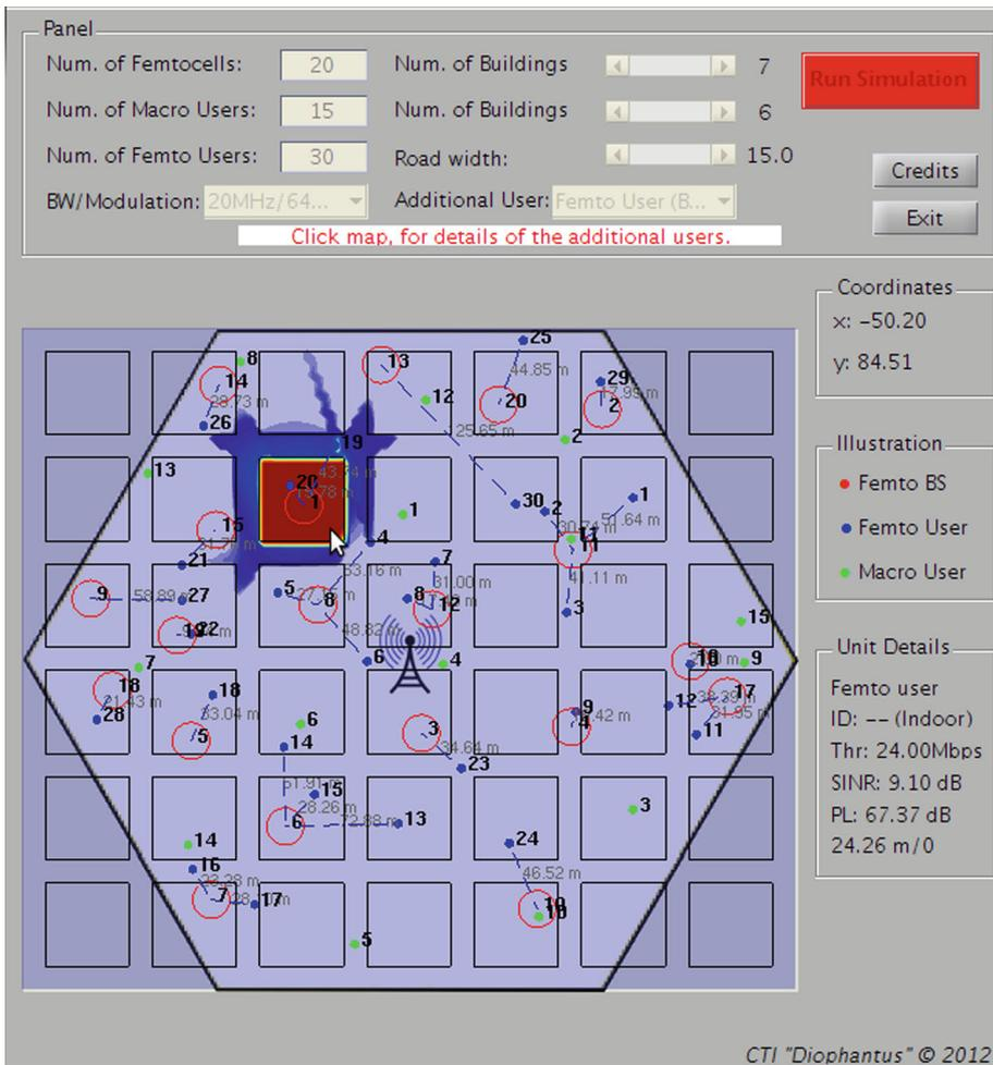
**Fig. 3** Example of the graphical presentation of the resulting performance
