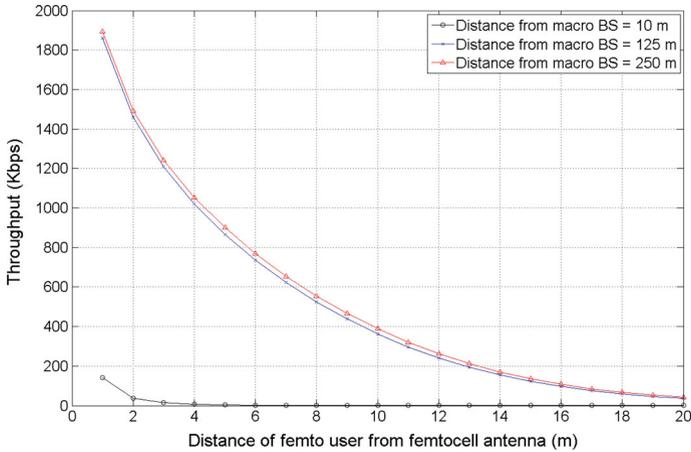
**Fig. 7** Throughput for an indoor femto UE against the distance from the femto BS when macrocell interference exists
