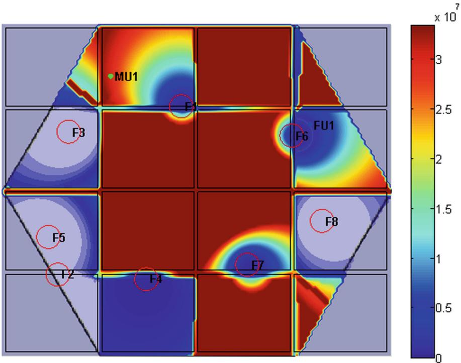
**Fig. 12** Data-rate map of IFR with femtocells utilizing the entire bandwidth
