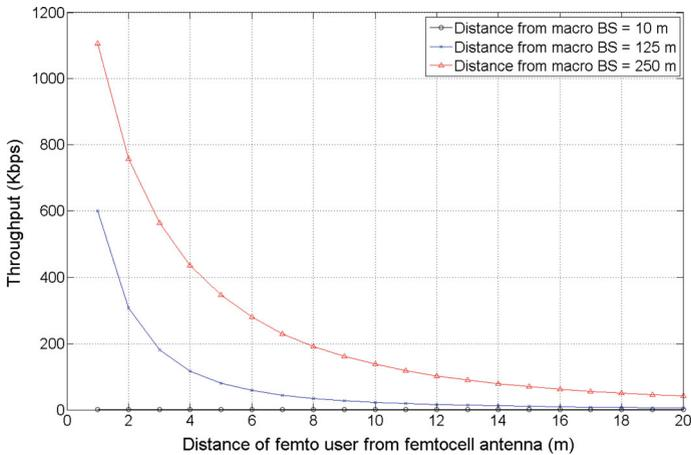
**Fig. 8** Throughput for an outdoor femto UE against the distance from the femto BS when macrocell interference exists
