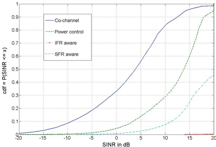
Fig. 17 CDF of SINR at cell’s borders for different scenarios
