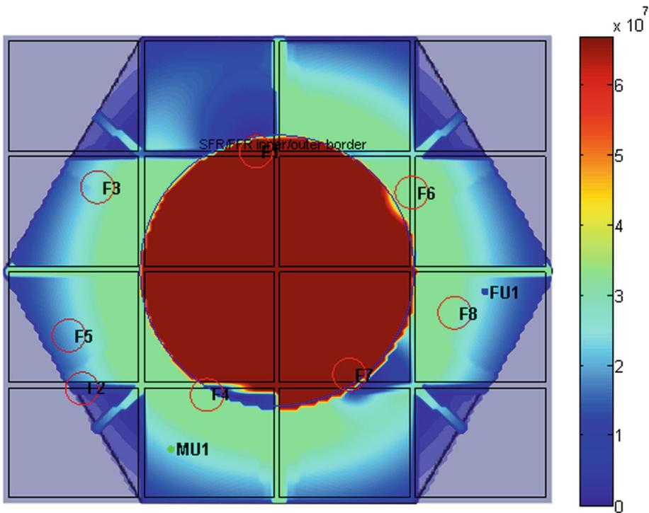
**Fig. 13** Data rate map of SFR with adapted femtocells
