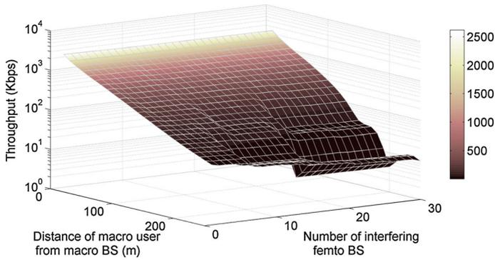
**Fig. 9** Throughput for a moving user against the distance from the macro BS and the number of femtocells
