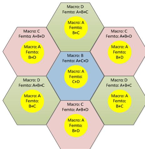
Fig. 2. Proposed frequency allocation for an integrated femtocell/macrocell environment
