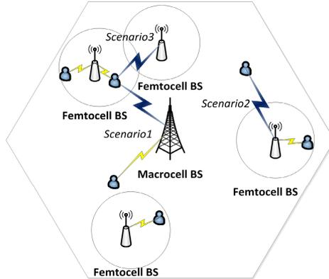
Fig. 1. Downlink interference scenarios in an integrated femtocell/macrocell environment
