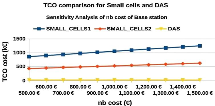
Fig. 3 The TCO comparison of both small cells and DAS deployments for  $C^{nb}$  SA
