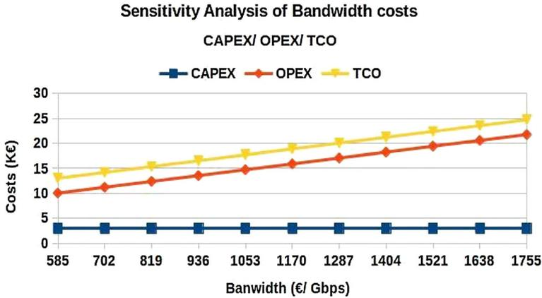
Fig. 10 The SA of DAS bandwidth costs  $f_{DAS}^{bw}$  for DAS CAPEX, OPEX and TCO
