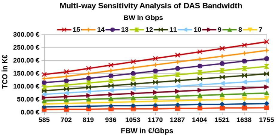
Fig. 16 The Multi-way SA of DAS overall cost  $C_{DAS}^{TCO}$  based on the allocated bandwidth
