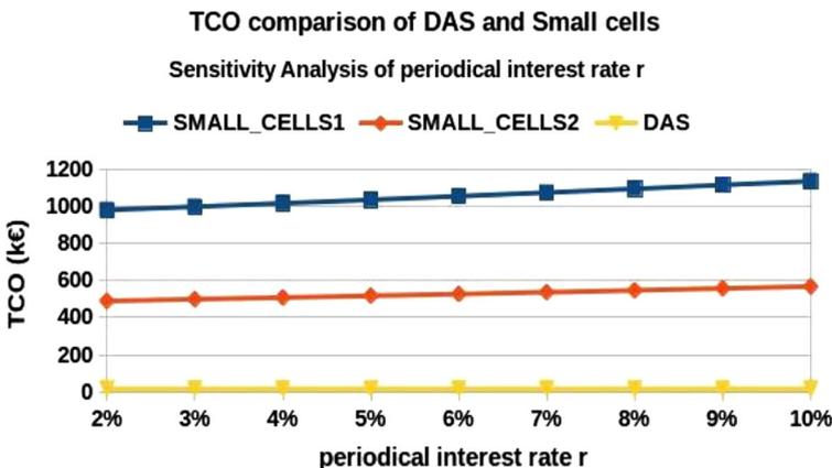
Fig. 5 The TCO comparison of both small cells and DAS deployments for the periodical interest rate  $r$  SA
