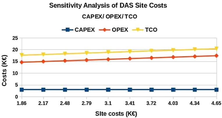
Fig. 8 The SA of DAS site costs  $c_{DAS}^s$  for DAS CAPEX, OPEX and TCO
