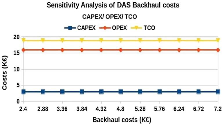
Fig. 12 The SA of DAS backhaul costs  $C_{DAS}^{bh}$  for DAS CAPEX, OPEX and TCO
