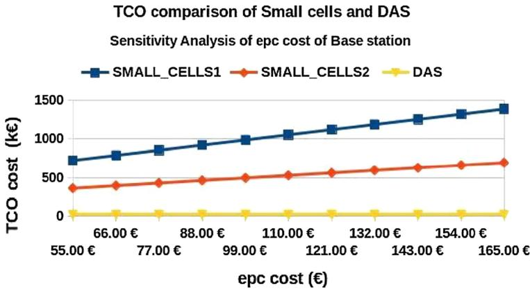
Fig. 4 The TCO comparison of both small cells and DAS deployments for  $C^{epc}$  SA
