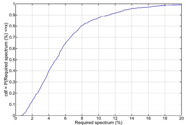
Fig. 3. Percentage of available spectrum required by the femto BS to maintain prior performance for non-CSG users.
