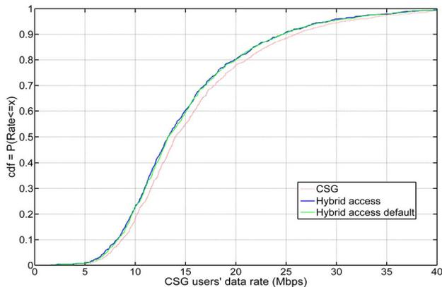
Fig. 4. CDF of CSG users throughput for the different access modes.
