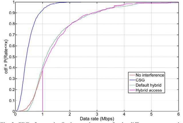
Fig. 2. CDF of non-subscribed users data rates for the different access modes.
