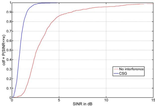
Fig. 1. CDF of MUEs' SINR before and after the deployment of CSG femtocells.
