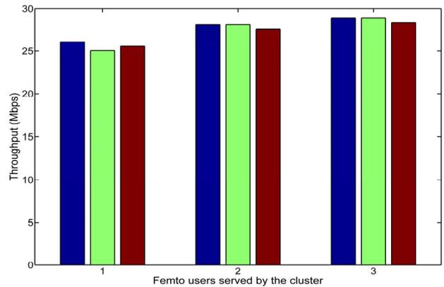
Fig. 5. Power control for 3 femto BS in a cluster. Femto BS 1 is the femtocell in hybrid access, and 2,3 are the neighbouring femtocells. The first column is the initial throughput, the second when hybrid access is employed and the third when the power control is enforced.
