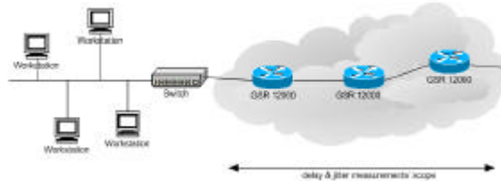
Fig. 3. Over-provisioning factor monitoring testbed
