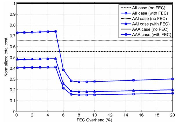
**Figure 3. Cost vs. FEC Overhead (Packet loss rate = 5%, UE population = 100).**
