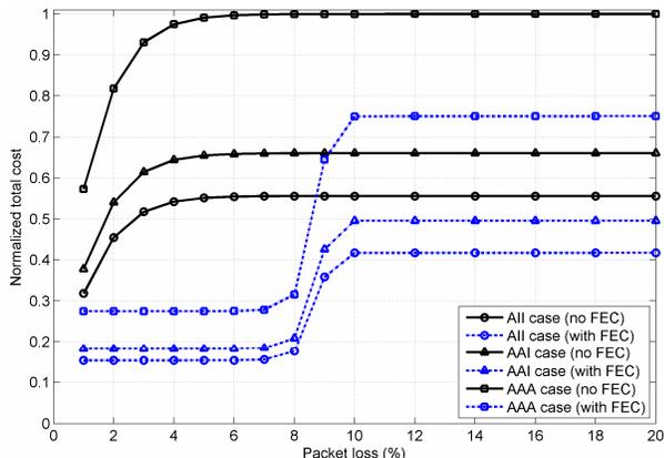
Figure 5. Cost vs. Packet loss rate (UE population = 100, FEC overhead = 10%).
