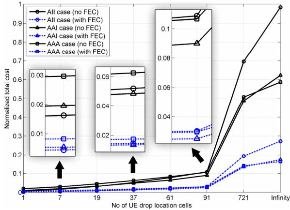
**Figure 1. Cost vs. MBSFN Deployment (Packet loss rate = 5%, FEC overhead = 10%, UE population = 100).**
