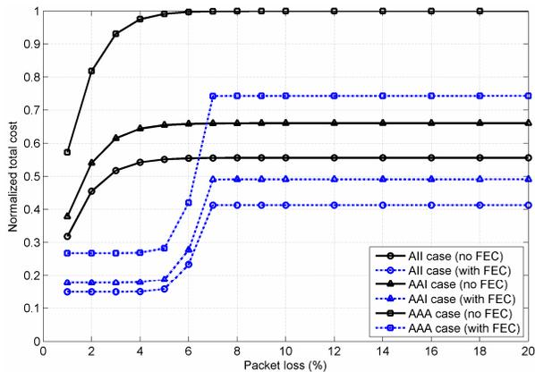
Figure 4. Cost vs. Packet loss rate (UE population = 100, FEC overhead = 7%).
