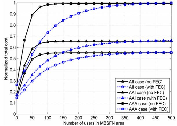
**Figure 2. Cost vs. Multicast User Population (Packet loss rate = 5%, FEC overhead = 5%).**
