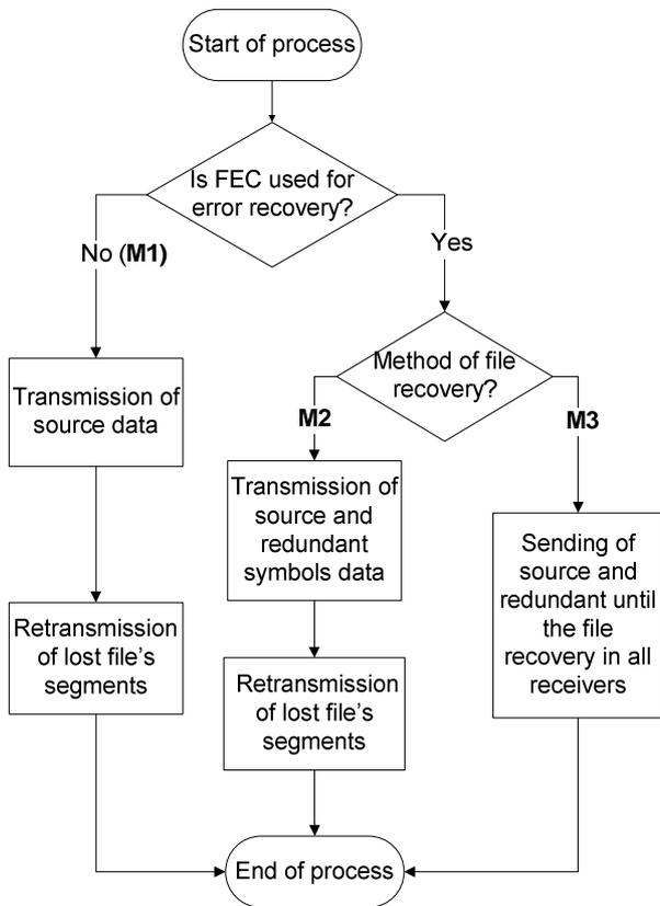
Figure 1. Flowchart of error recovery methods.
