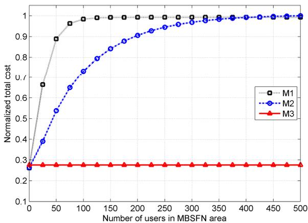
Figure 5. Cost vs. multicast user population (packet loss rate=5%, fixed FEC overhead = 5%).
