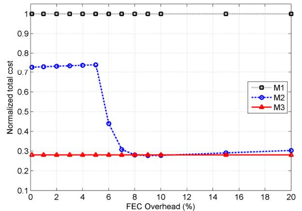
Figure 4. Cost vs. fixed FEC overhead (packet loss rate = 5%, UE population = 100)
