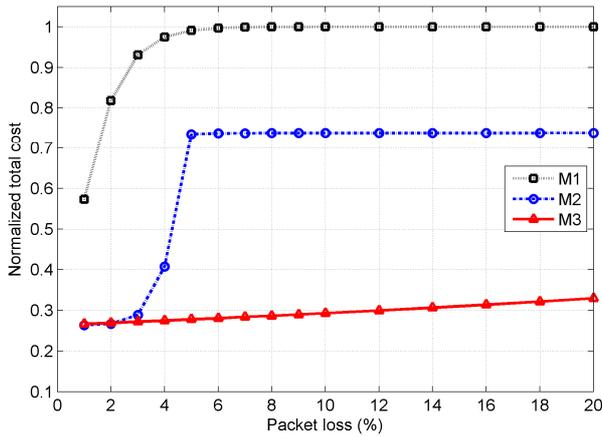
Figure 2. Cost vs. packet loss rate (UE population = 100, fixed FEC overhead = 5%).
