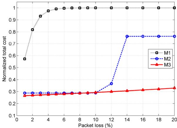
Figure 3. Cost vs. packet loss rate (UE population = 100, fixed FEC overhead=15%).
