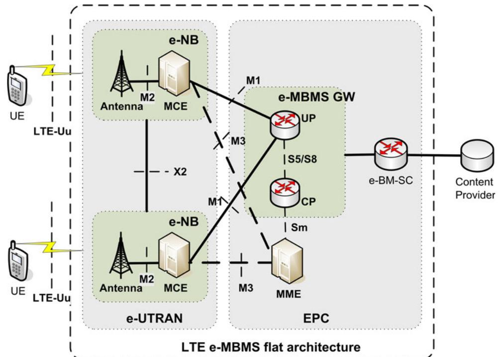
which is external to the network. An e-BM-SC serves all the e-MBMS GWs in a network.
