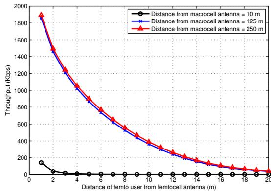
Fig. 3. Throughput for an indoor femto user against the distance from the femto BS when macrocell interference exists.
