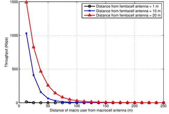
Fig. 1. Throughput for an indoor macro user against the distance from the macro BS when femtocell interference exists.
