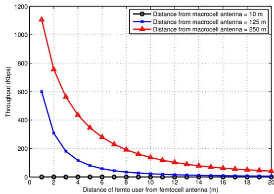
Fig. 4. Throughput for an outdoor femto user against the distance from the femto BS when macrocell interference exists.
