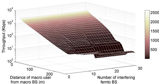
Fig. 6. Throughput for a moving user against the distance from the macro BS and the number of femtocells.
