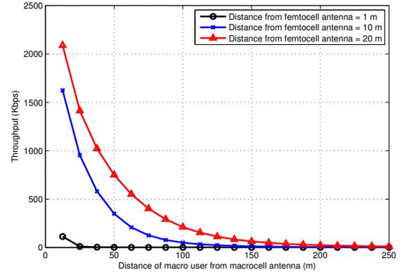
Fig. 2. Throughput for an outdoor macro user against the distance from the macro BS when femtocell interference exists.
