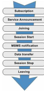
Fig. 2. Phases of MBMS multicast service provision
