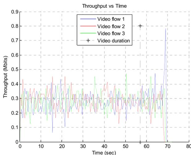
Figure 8. Bandwidth usage for three videos transmission without MIMC support.
