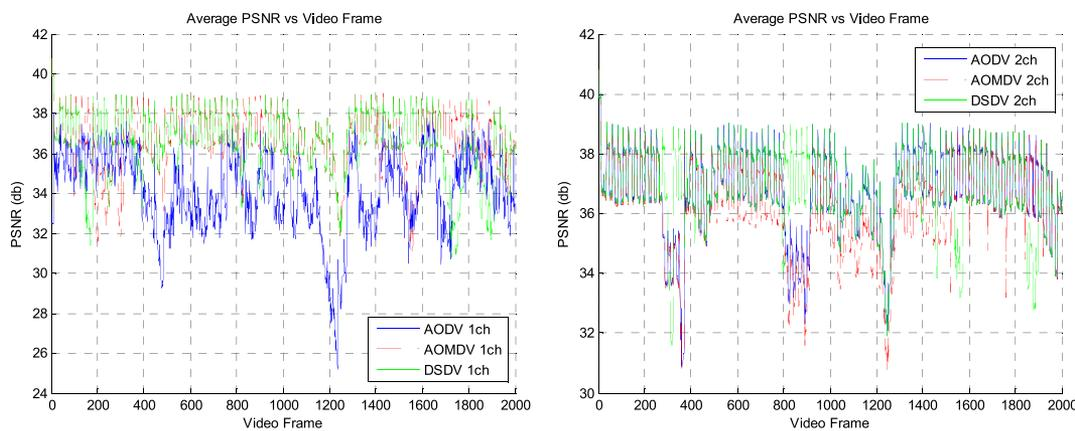
Figure 24. Average PSNR without (left) and with (right) MIMC for topology 2.
