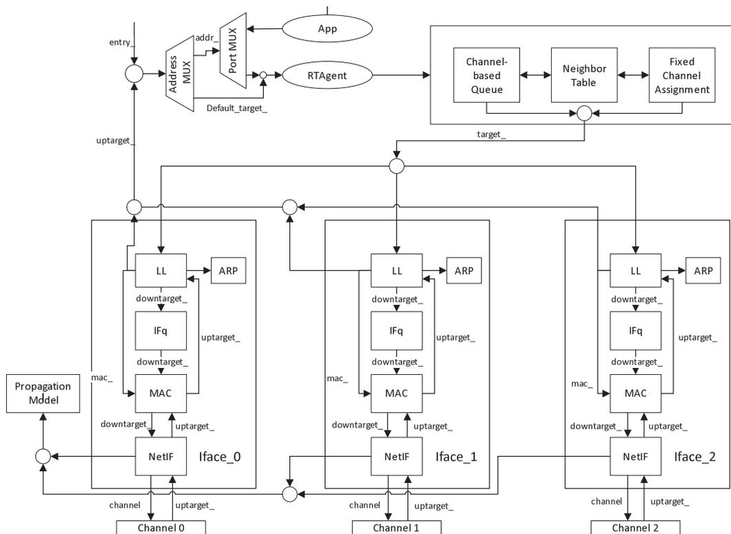
Figure 3. Mobile node architecture, with multiple interface support.
