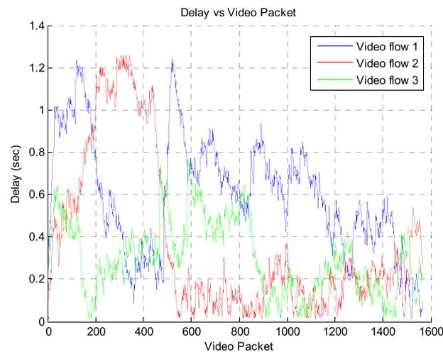
Figure 14. Delay for three videos transmission with rate adaptation.
