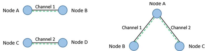
Figure 5. Usage of multiple channels and multiple interfaces for different links.
