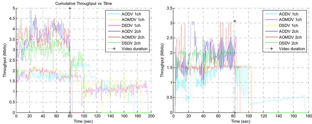
Figure 20. Cumulative bandwidth for topology 1 (left) and 2 (right).
