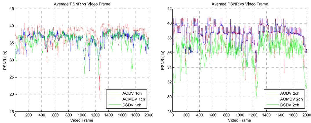
Figure 23. Average PSNR without (left) and with (right) MIMC for topology 1.
