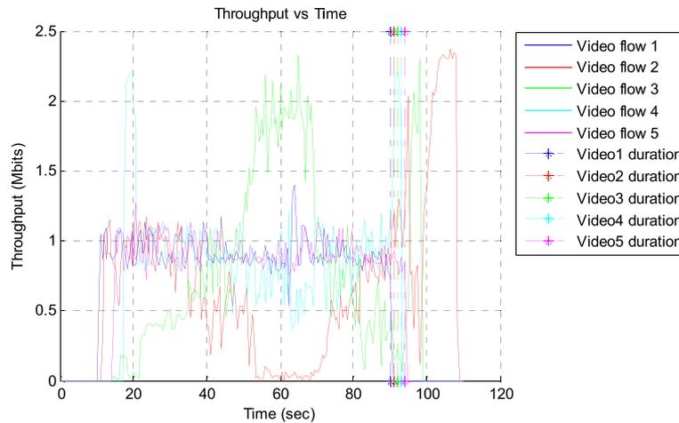
Figure 26. Throughput of the video streams in the case of AODV with MIMC.
