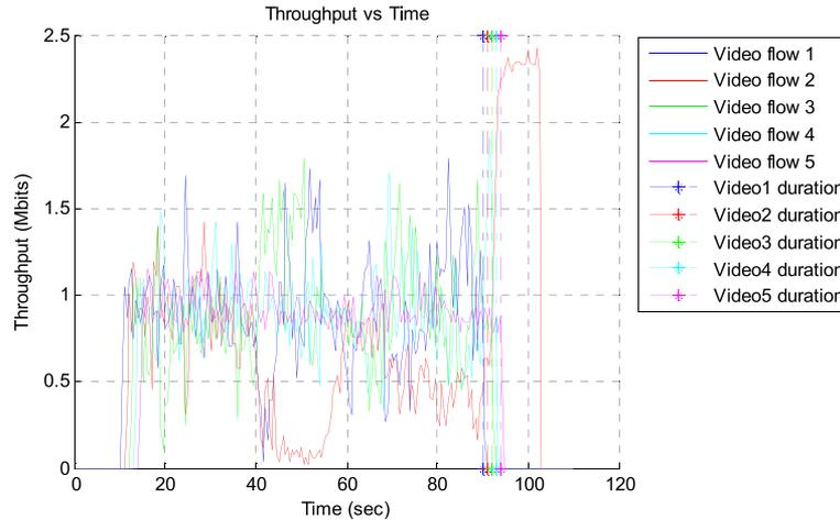
Figure 27. Throughput of the video streams in the case of AODV with the proposed mechanism.
