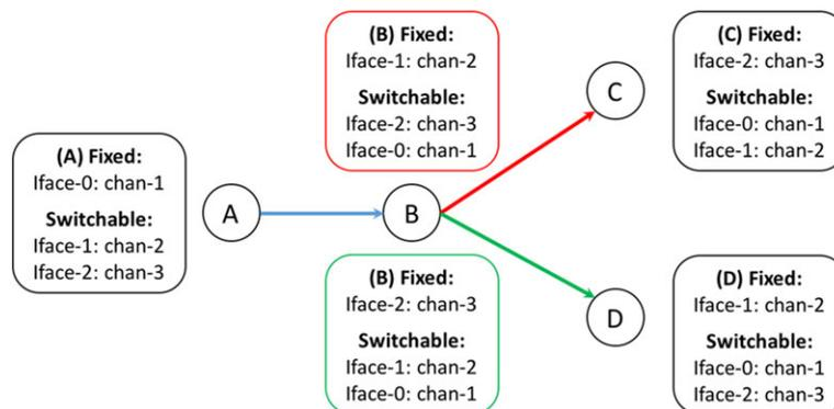
Figure 6. Fixed and switchable interfaces example for four nodes with three interfaces each.
