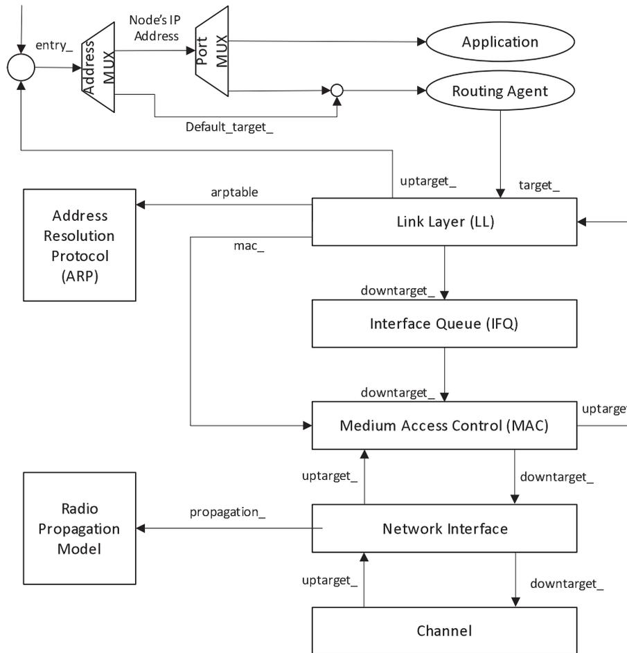
Figure 2. Default mobile node architecture.
