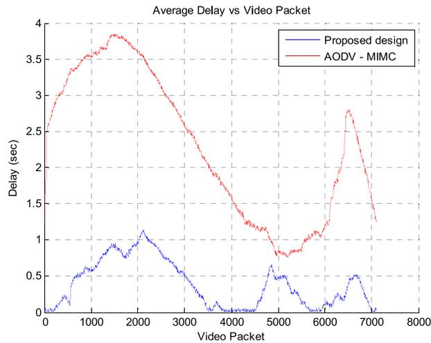
Figure 31. Average delay comparison per packet with and without the proposed mechanism.
