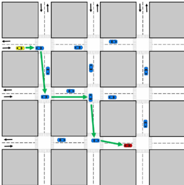
Figure 5. Multi-hop route from source (yellow node) to destination (red node). Nodes moving in road intersections function as route connectors
