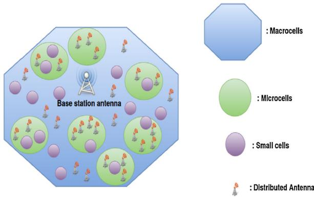
**Fig. 1** The suggested deployment for DAS and small cells
