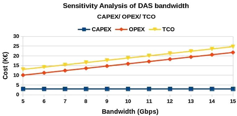
Fig. 9 The SA of DAS bandwidth costs  $bw_{DAS}$  for DAS CAPEX, OPEX and TCO
