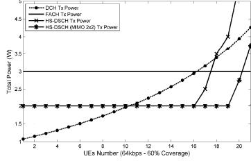
Figure 2. MBMS Power Allocation, 64Kbps, 60% coverage
