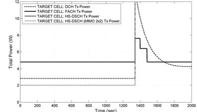
Figure 7. Target Cell: Output of power level computation phase
