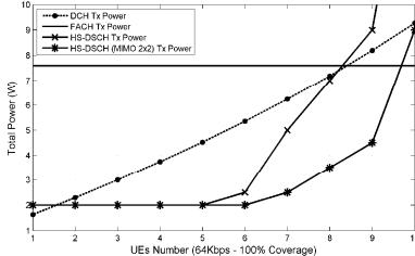
Figure 4. MBMS Power Allocation, 64Kbps, 100% coverage
