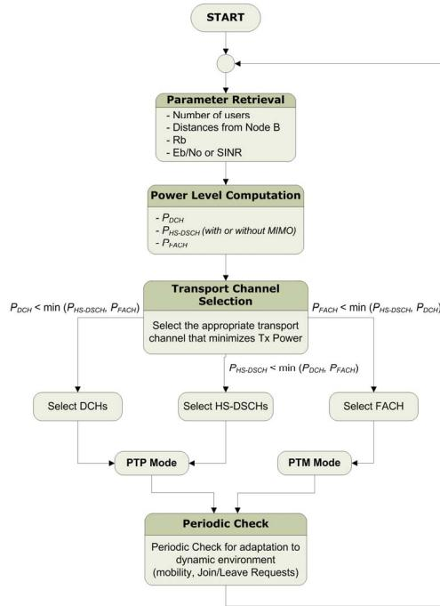
Figure 1. Power Counting Scheme with MIMO functionality
