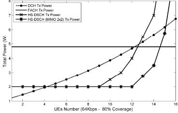
Figure 3. MBMS Power Allocation, 64Kbps, 80% coverage
