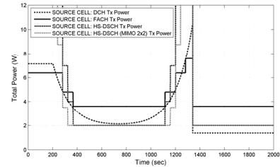
Figure 6. Source Cell: Output of power level computation phase
