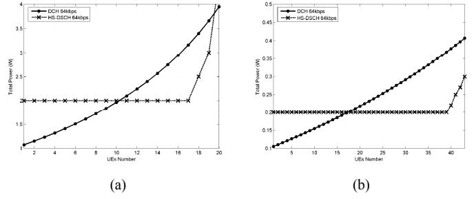
Figure 3. MBMS Tx Power 64Kbps, 60% coverage (a) Macrocell, (b) Microcell.
