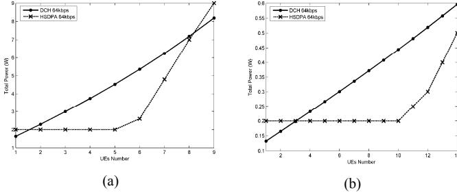
Figure 5. MBMS Tx Power 64Kbps, 100% coverage (a) Macrocell, (b) Microcell.
