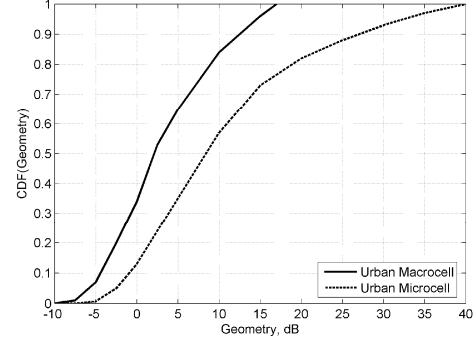
Figure 2. Geometry CDF Macrocell – Microcell.
