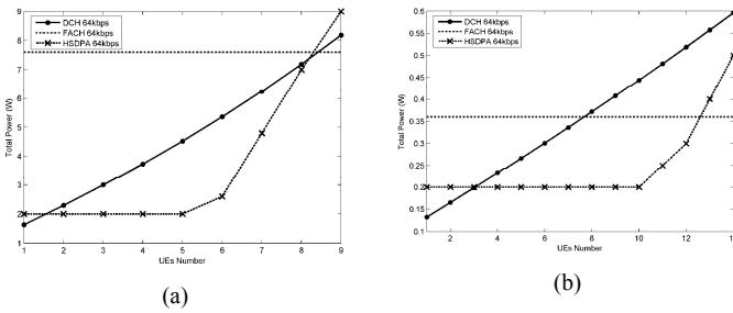
Figure 6. MBMS Power Allocation 64Kbps, 100% coverage (a) Macrocell, (b) Microcell.
