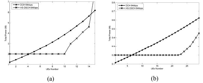
Figure 4. MBMS Tx Power 64Kbps, 80% coverage (a) Macrocell, (b) Microcell.
