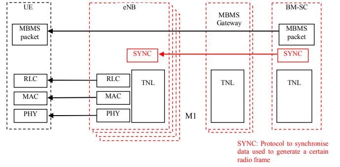
Figure 4. Content synchronization in MBSFN.
