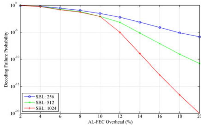
Figure 10. Raptor FEC decoding failure probability versus AL-FEC overhead.
