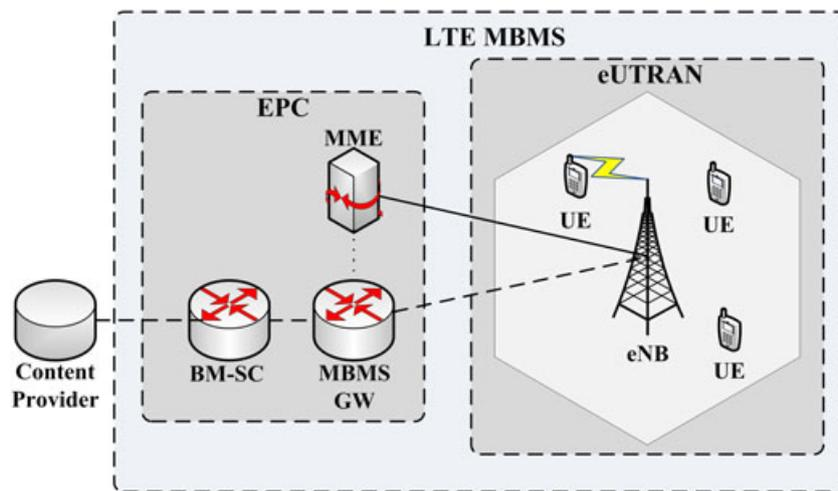
Figure 2. LTE MBMS network architecture.
