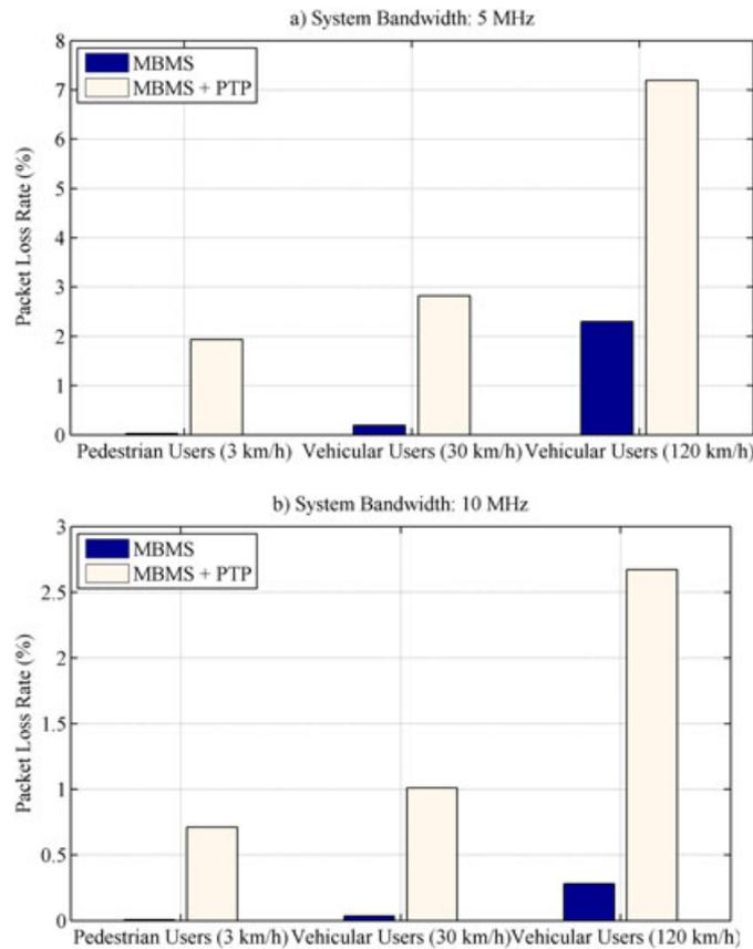
Figure 5. Packet loss rate versus different mobility models for system bandwidth (a) 5 MHz and (b) 10 MHz.
