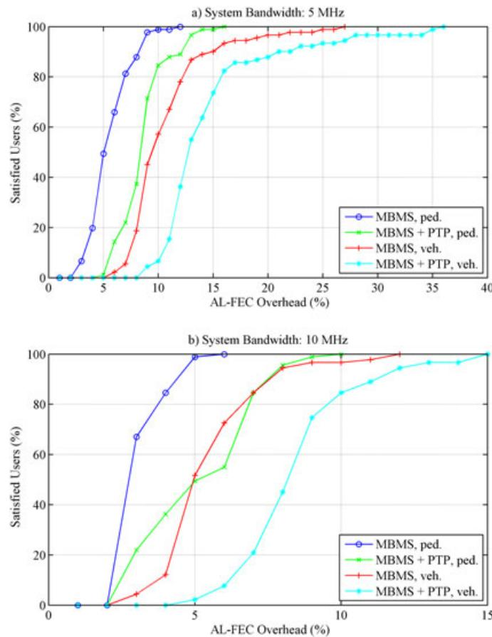
Figure 8. Percentage of satisfied users versus AL-FEC overhead for system bandwidth: (a) 5 MHz and (b) 10 MHz.
