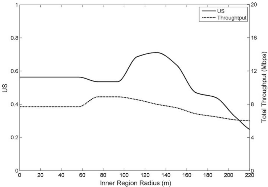
Fig. 5 US and cell total throughput versus inner region radius (inner region RBs = 2)
