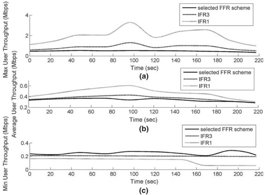
**Fig. 10** a Maximum, b average and c minimum user throughput versus time for the three schemes
