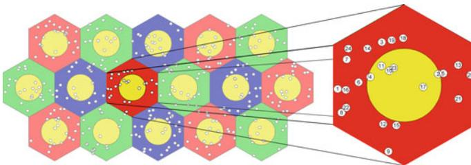
**Fig. 3** Optimal FFR scheme selected by the mechanism (inner region radius = 131 m)
