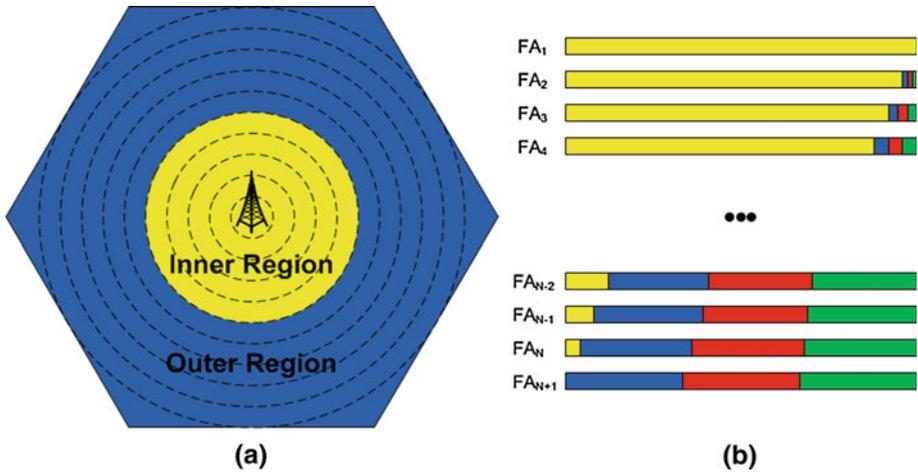
Fig. 2 a Cell division and b frequency allocations of the mechanism
