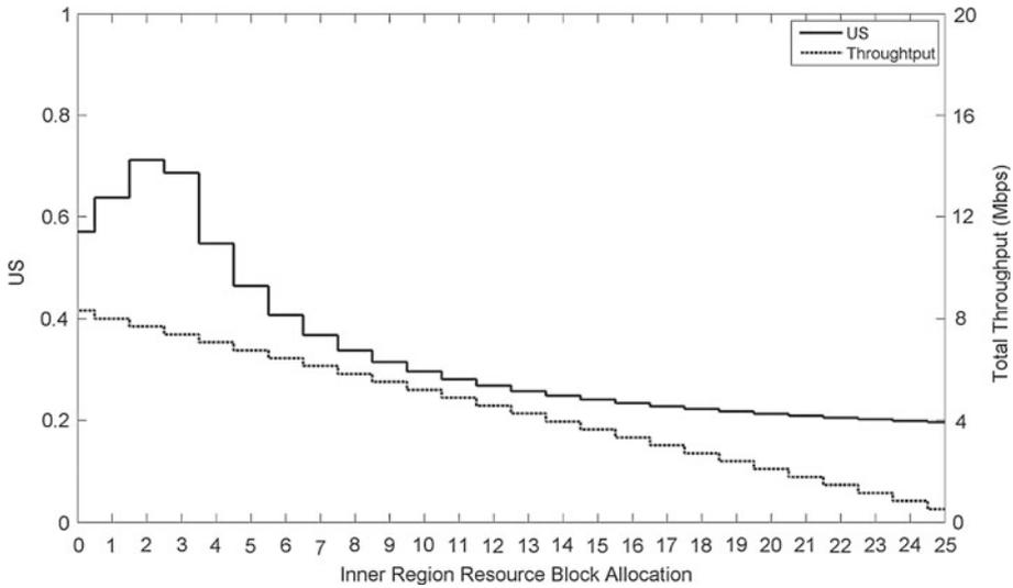
Fig. 4 US and cell total throughput versus inner region RB allocation (inner region radius = 131 m)
