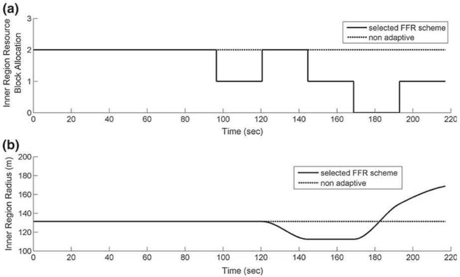
**Fig. 7** **a** Inner region RBs’ allocation and **b** inner region radius versus time with and without the adaptation process
