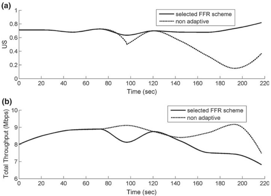
**Fig. 8** a US and b cell total throughput versus time with and without the adaptation process
