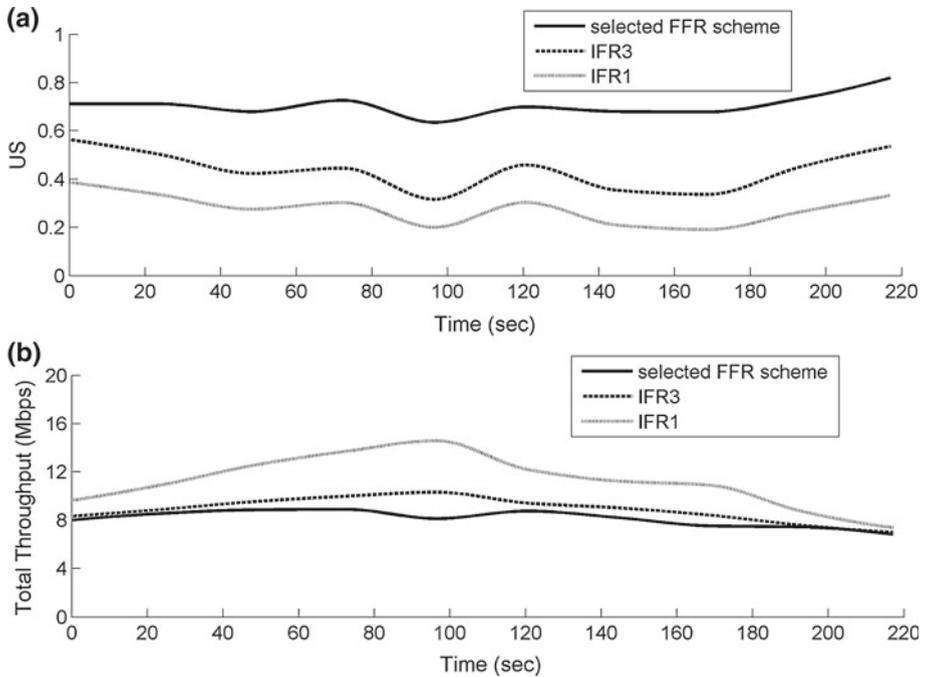
**Fig. 9** a US and b cell total throughput comparison of the three schemes (IFR1, IFR3 and selected FFR scheme)
