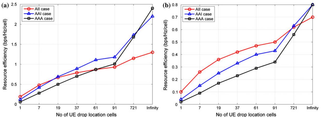
Fig. 3 Resource efficiency versus number of UE drop location cells for: a ISD = 500 m (macro Case 1), b ISD = 1732 m (macro Case 3)
