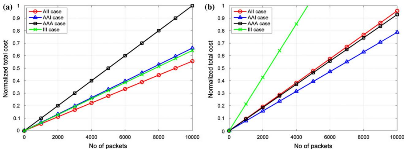
**Fig. 5** MBSFN cost for AII, AAI, AAA versus number of packets for macro Case 1 when  $k_{air} = 0.9$  and **a** UE drop location cells = 7, **b** UE drop location cells = 91
