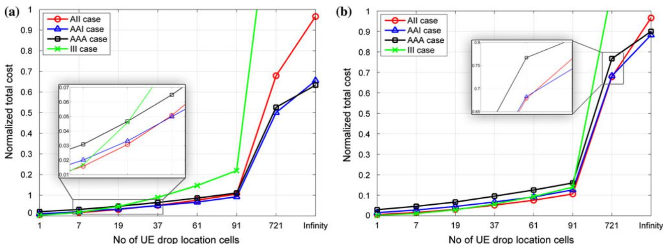
**Fig. 7** MBSFN cost for AII, AAI, AAA versus number of UE drop location cells when  $k_{air} = 0.8$  for: **a** ISD = 500 m (macro Case 1), **b** ISD = 1,732 m (macro Case 3)
