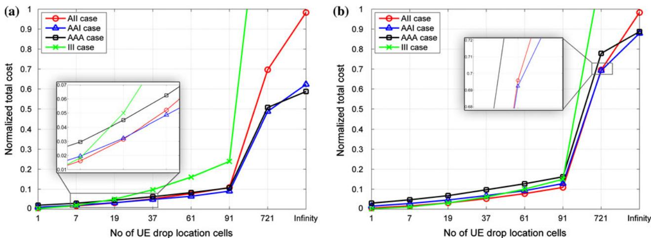
**Fig. 6** MBSFN cost for AII, AAI, AAA versus number of UE drop location cells when  $k_{air} = 0.9$  for: **a** ISD = 500 m (macro Case 1), **b** ISD = 1,732 m (macro Case 3)
