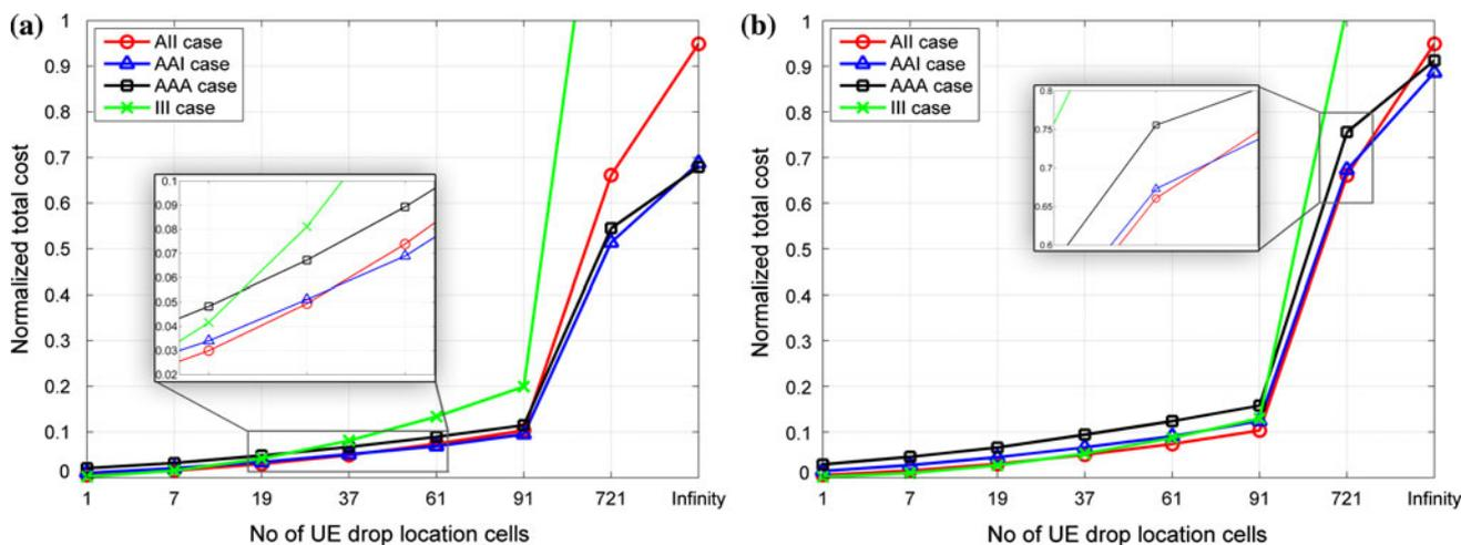
**Fig. 8** MBSFN cost for AII, AAI, AAA versus number of UE drop location cells when  $k_{air} = 0.7$  for: **a** ISD = 500 m (macro Case 1), **b** ISD = 1,732 m (macro Case 3)
