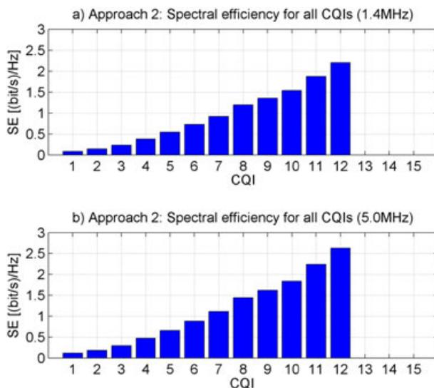
Figure 5. SE for all CQIs (second approach) for: (a) 1.4 MHz and (b) 5.0 MHz.
