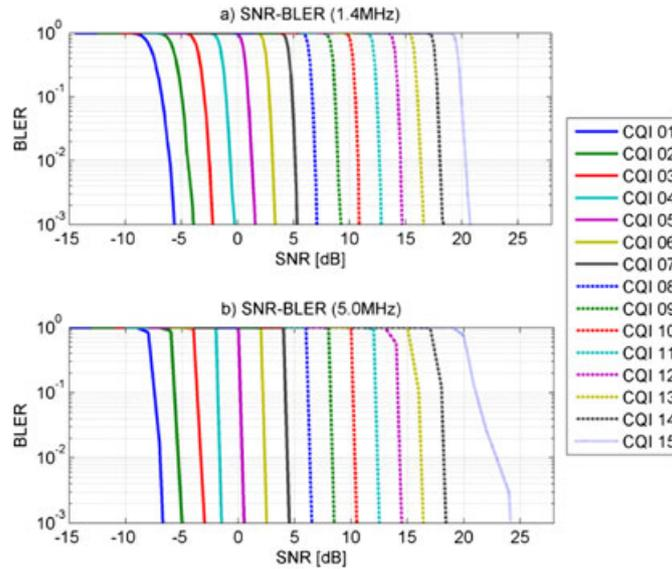
Figure 1. SNR–BLER curves obtained for: (a) 1.4 MHz and (b) 5.0 MHz.
