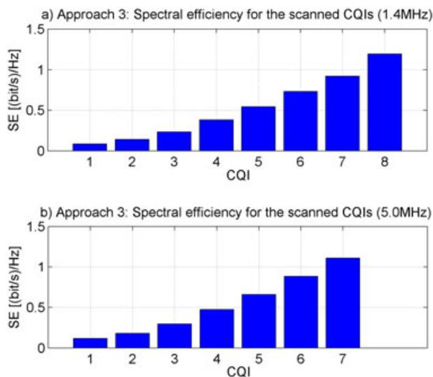
Figure 6. SE only for the CQIs scanned to reach the SE target over the area (third approach) for: (a) 1.4 MHz and (b) 5.0 MHz.
