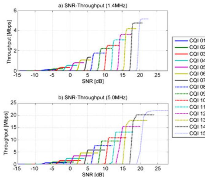
Figure 3. Throughput for all CQIs obtained for: (a) 1.4 MHz and (b) 5.0 MHz.
