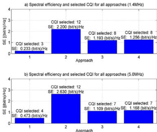
Figure 8. SE evaluation and CQI selection predefined number of users for: (a) 1.4 MHz and (b) 5.0 Mhz.
