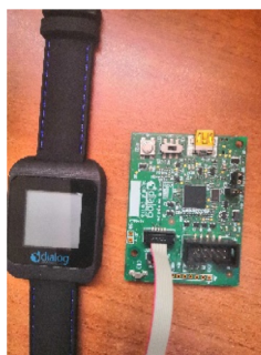
Fig. 3. The DA 14861 prototype with the jtag debugger.
