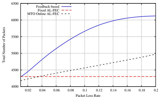
Fig. 3: Total Number of Packets vs. Packet Loss Rate
