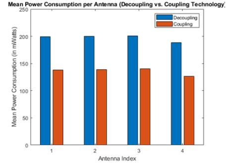
Fig.4.Comparison Energy Consumption for 500 UEs in Micro BSs
