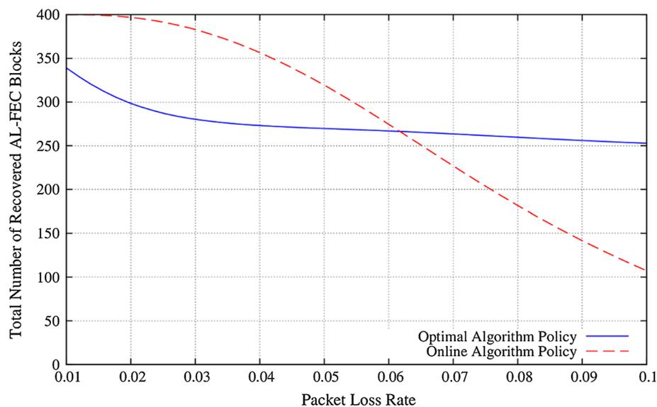
**Fig. 2** Average number of recovered source blocks per user versus packet loss rate
