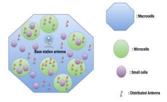
Fig. 1 The suggested deployment for DAS and small cells
