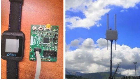
Fig. 3. MultiTech Conduit LoRa Gateway located in the University of Patras
