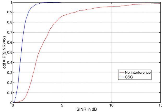
Fig. 1. CDF of MUEs' SINR before and after the deployment of CSG femtocells.
