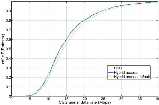
Fig. 4. CDF of CSG users throughput for the different access modes.
