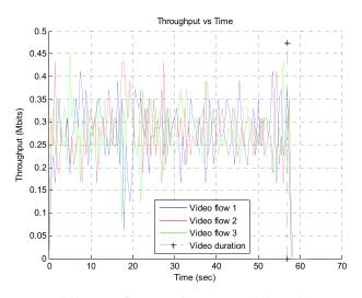
Figure 12. Bandwidth usage for three videos transmission with rate adaptation.
