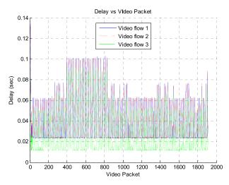
Figure 11. Delay for three videos transmission with MIMC support.
