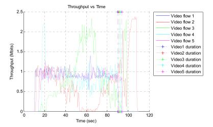
Figure 26. Throughput of the video streams in the case of AODV with MIMC.
