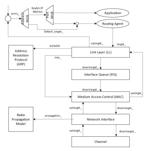
Figure 2. Default mobile node architecture.
