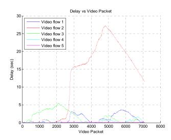
Figure 30. Packet delay of the video streams in the case of AODV with the proposed mechanism.
