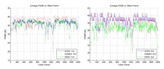
Figure 23. Average PSNR without (left) and with (right) MIMC for topology 1.
