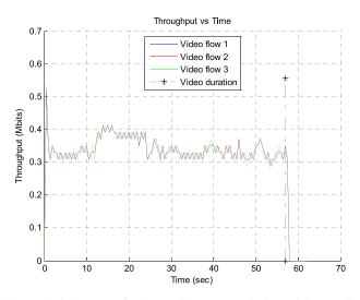
Figure 10. Bandwidth usage for three videos transmission with MIMC support.
