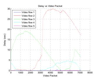
Figure 29. Packet delay of the video streams in the case of AODV with MIMC.
