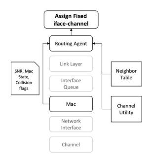
Figure 7. Interface switching mechanism.
