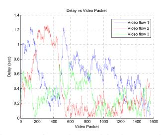
Figure 14. Delay for three videos transmission with rate adaptation.
