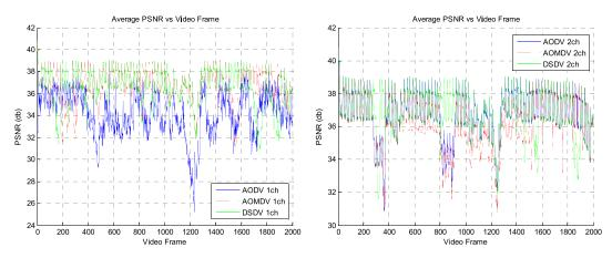
Figure 24. Average PSNR without (left) and with (right) MIMC for topology 2.
