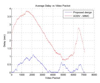
Figure 31. Average delay comparison per packet with and without the proposed mechanism.
