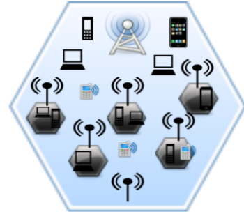
Fig. 1: The proximity of the cells in Ultra-dense deployment. Letting the cell-to-cell distance=10m and the cell radius=10m.
