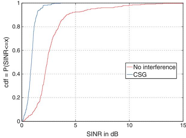
Figure 1. CDF of macrocell users signal to interference plus noise ratio (SINR) before and after the deployment of closed subscriber group (CSG) femtocells.
