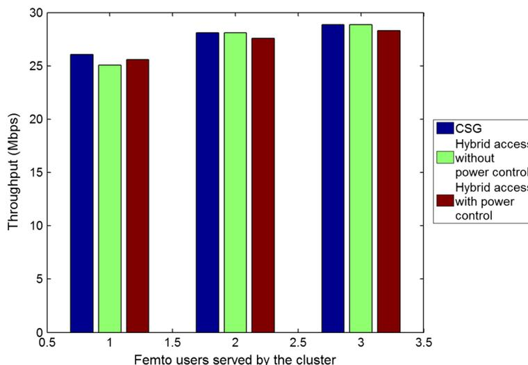
Figure 5. Capacity of closed subscriber group (CSG) users without including  $IMP$  parameter.
