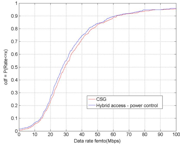
Figure 7. Comparison of overall capacity of the two approaches. CSG, closed subscriber group.
