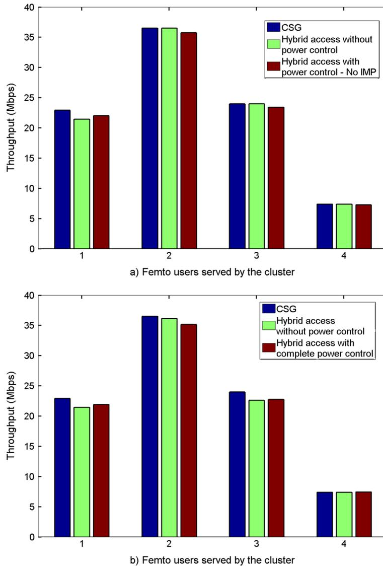
Figure 6. Capacity of closed subscriber group (CSG) users without (a) and including (b) *IMP* parameter.
