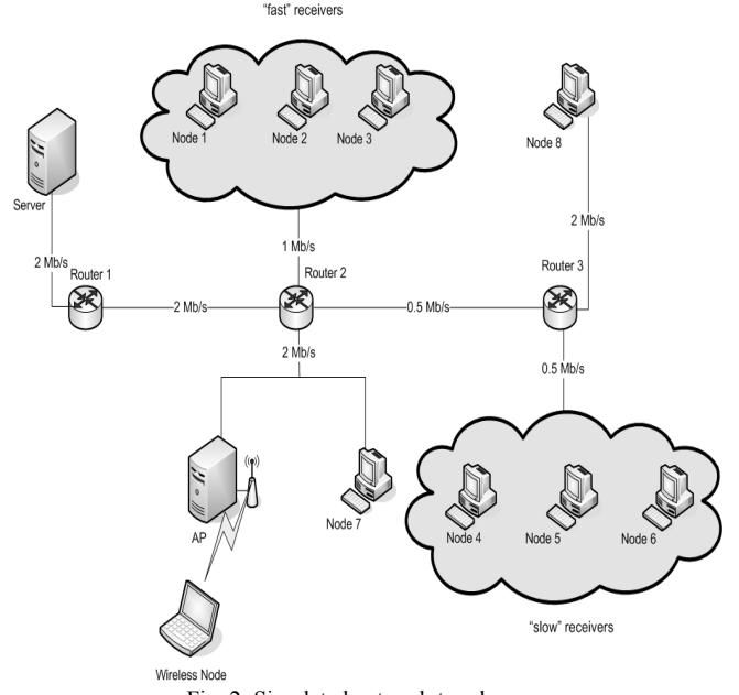
Fig. 2. Simulated network topology
