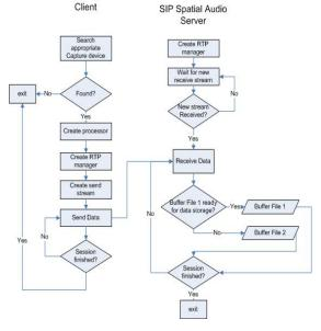
Figure 5: RTP streaming flowchart.
