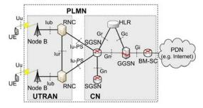
Figure 1. UMTS architecture for MBMS service.
