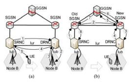
Figure 3. User mobility handling: (a) inter-RNS handover and (b) inter-SRNS relocation.
