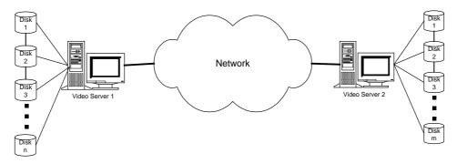
Figure 3. The disk storage architecture
