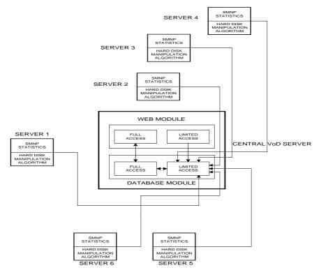
Figure 1. The system's modules
