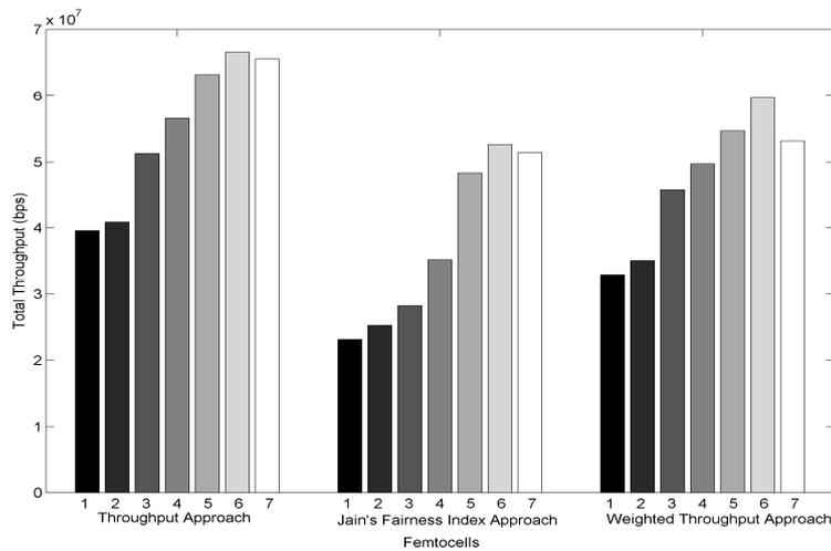
Fig. 7. Total throughput for each femtocell added to the topology
