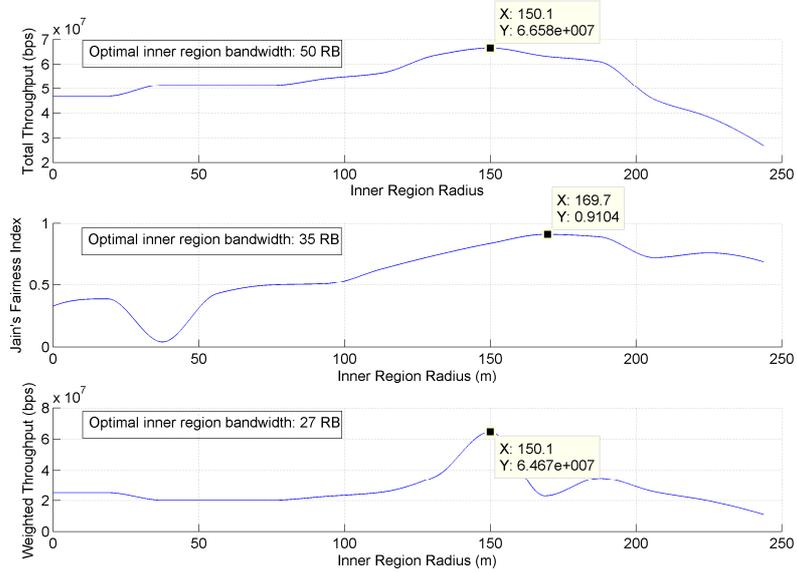
**Fig. 4.** Selection of optimal inner region radius
