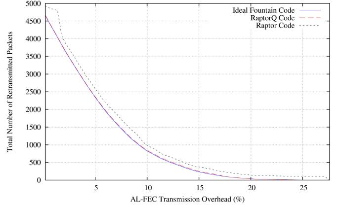
Fig. 4. Total Number of Retransmitted Packets vs. AL-FEC Transmission Overhead
