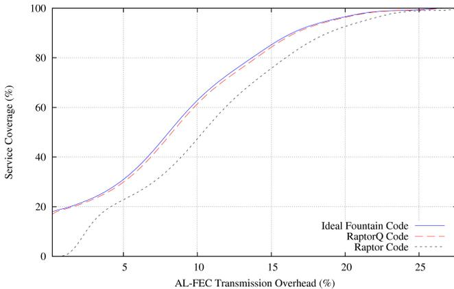
Fig. 3. Service Coverage vs. AL-FEC Transmission Overhead
