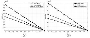
Figure 3: Total cost in function of  $\alpha$ ,  $\delta$ =3000 for (a) macrocell, (b) microcell.
