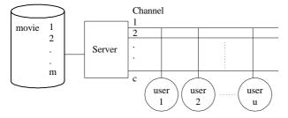
Figure 2: The model of a VOD system.
