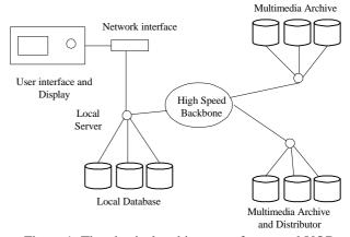
Figure 1: The physical architecture of a general VOD system.
