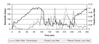
Figure 4. Video transmission rate and packet loss rate during experiment one.
