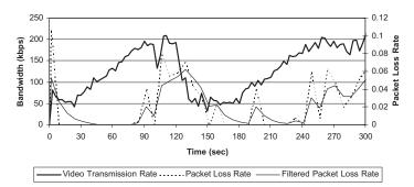
Figure 8. Video transmission rate and packet loss rate during experiment two with  $R_{\text{decrease}} = 0.5$ .
