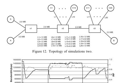
Figure 13. Server bandwidth, UDP-receiver bandwidth and IRF function values of simulation two.
