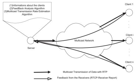
Figure 3. Multicast operation of the adaptive transmission mechanism.
