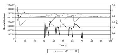
Figure 15. Server bandwidth, TCP source bandwidth and IRF function values of simulation three.
