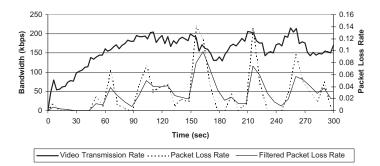
Figure 6. Video transmission rate and packet loss rate during experiment two with  $R_{decrease} = 0.85$ .
