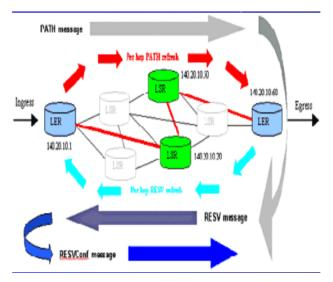
Figure 3 RSVP-TE operation for LSP establishment
