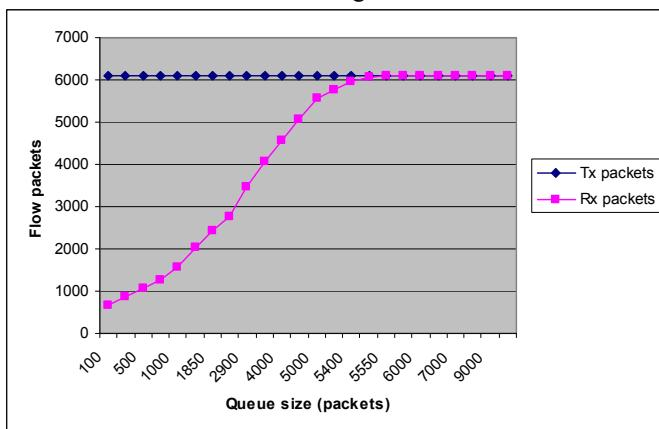
Figure 4 Flow behavior according to the size of the buffer
