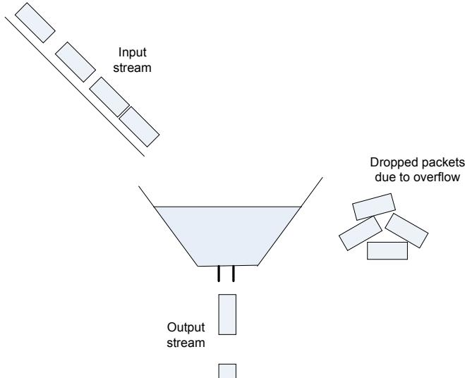
Figure 1 Leaky bucket operation
