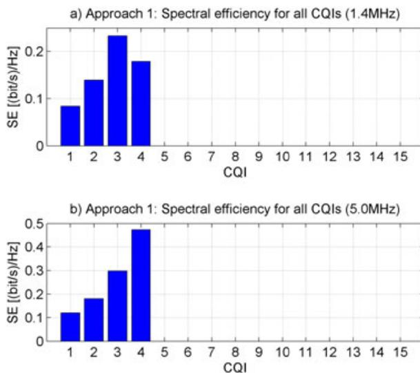
Figure 4. SE of the user with the lowest SINR for all CQIs (first approach) for: (a) 1.4 MHz and (b) 5.0 MHz.
