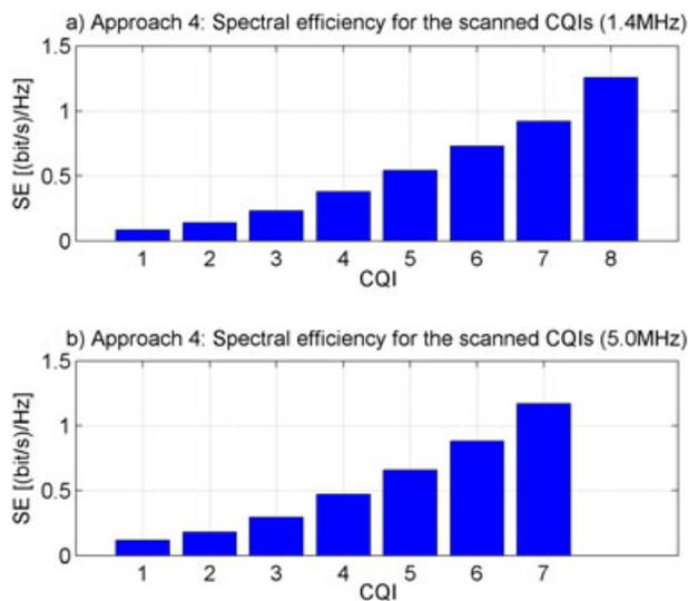
Figure 7. SE only for the CQIs scanned to reach the per-user SE target (fourth approach) for: (a) 1.4 MHz and (b) 5.0 MHz.
