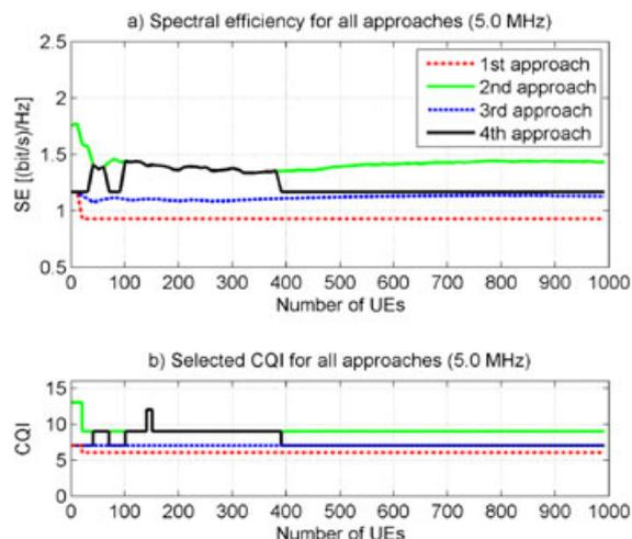
Figure 10. SE evaluation and CQI selection for variable number of users for 5.0 Mhz.
