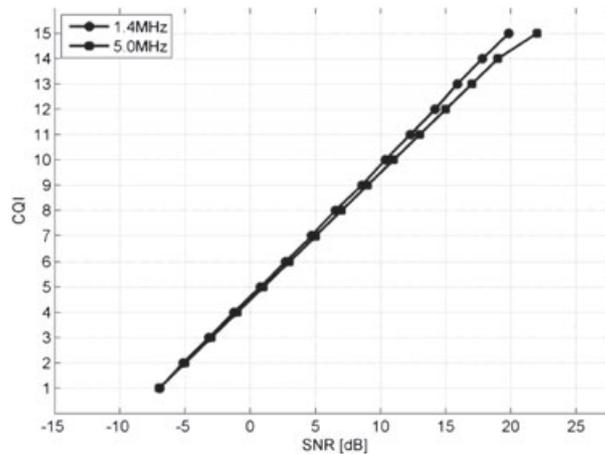
Figure 2. SINR to CQI mapping.
