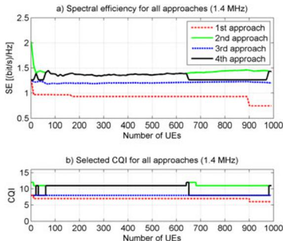
Figure 9. SE evaluation and CQI selection for variable number of users for 1.4 MHz.
