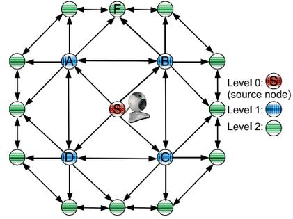
Figure 4. P2P topology.  $S$  is the source peer.
