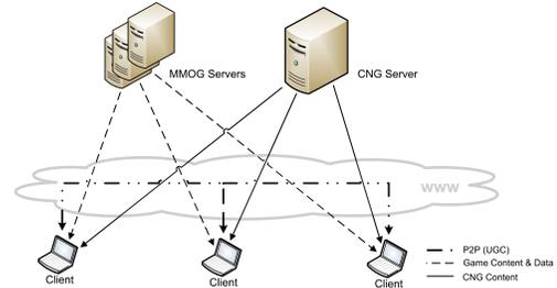
Figure 1. CNG architecture.
