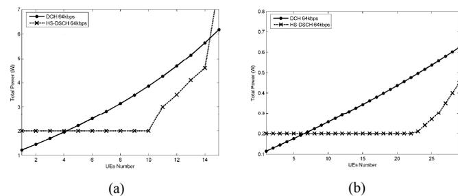
Figure 4. MBMS Tx Power 64Kbps, 80% coverage (a) Macrocell, (b) Microcell.
