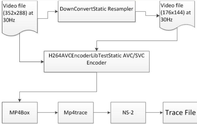
Figure 4. Simulation procedure
