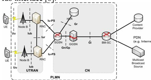
Figure 1: Release 6 UMTS Architecture.
