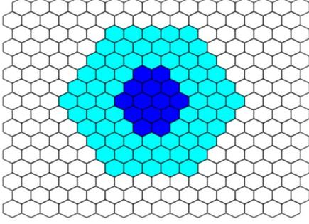
Figure 2. MBSFN area consisting of the centre cells and three assisting rings.
