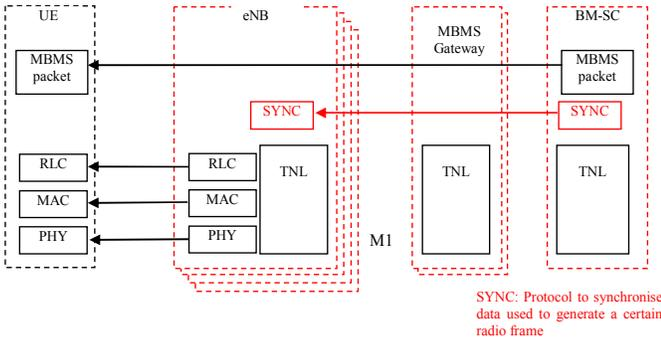
Figure 3. Content synchronization in MBSFN.
