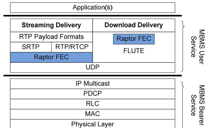
Figure 2. MBMS protocol stack.
