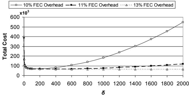
Figure 5. Total cost against  $\delta$  when  $p_{loss} = 5\%$  and  $\alpha = 0.9$ .
