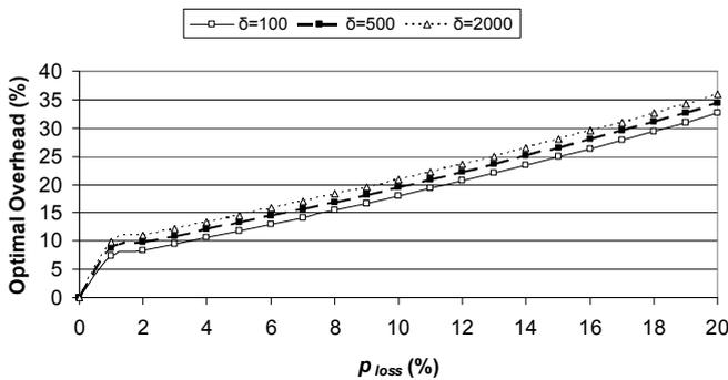
Figure 6. Optimal overhead against packet loss rate when  $\alpha = 0.1$ .
