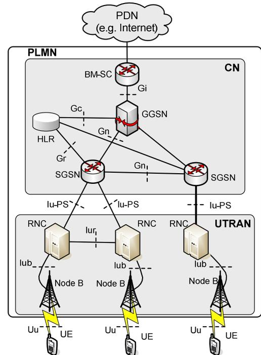
Figure 1. UMTS architecture for MBMS.
